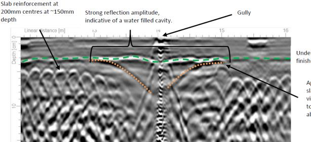
Underside of screed/surface finishes at ~80mm depth.
